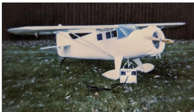
1987—1/4 scale Mr. Mulligan built by Lew Parish. 108" wingspan, 2.5 horsepower motor.
