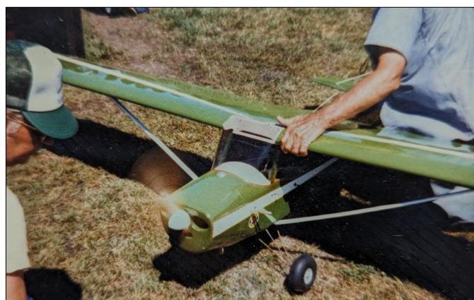
1984—Bud Nosen Champ. 108" wingspan, Quadra .35 motor, monocote covering. Seventeen pounds.
